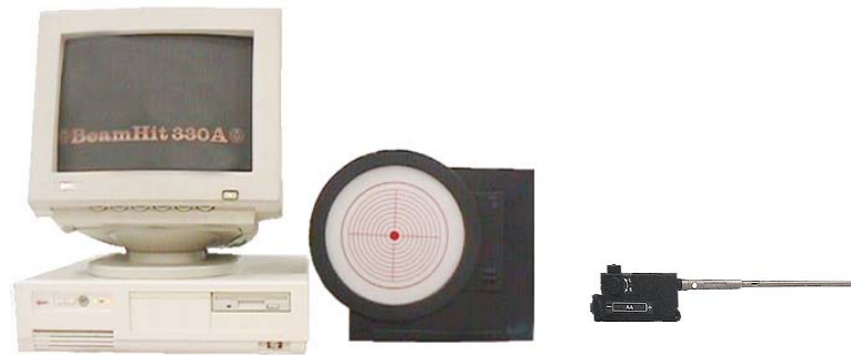
Figure 1. LMTS computer/monitor, sample electronic target, and laser transmitter with attached mandrel.
